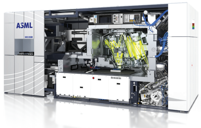
FIGURE 2. The ASML® TWINSKAN® NXE:3350B production-ready EUV system produces 125 computer wafers per hour using 13.5 nm wavelength light. It must keep a perfect vacuum while moving wafers at high speeds and loads, maintaining distortions to less than 1 nm.
