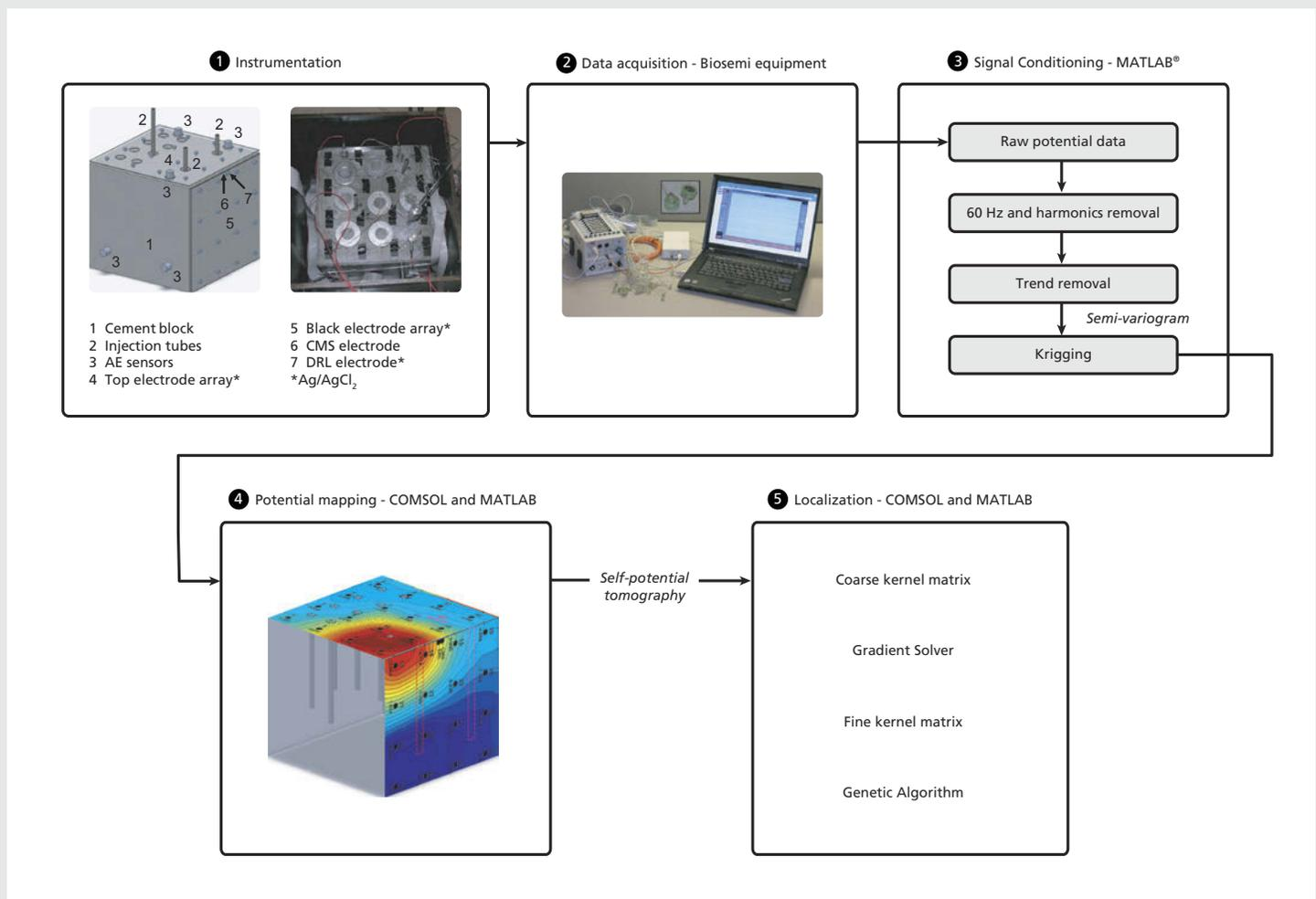
**FIGURE 2:** Flow chart for the processing of the electrical data. (1) Instrumentation of the porous cement block, (2) Data acquisition system, (3) Signal conditioning of the raw data, (4) Mapping the voltage response using ordinary krigging (geostatistical inferences), (5) Localization of the causative sources in the block.
