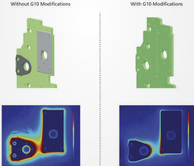
**FIGURE 3:** Dielectric stress simulation of G10 board with mounting plates for switching assemblies. During a tap change, there is a high voltage between the mounting plates. The simulation plots show the results with and without geometry modifications of the G10 board. These modifications significantly reduce the dielectric stress on the board, as shown in the simulation on the right.
