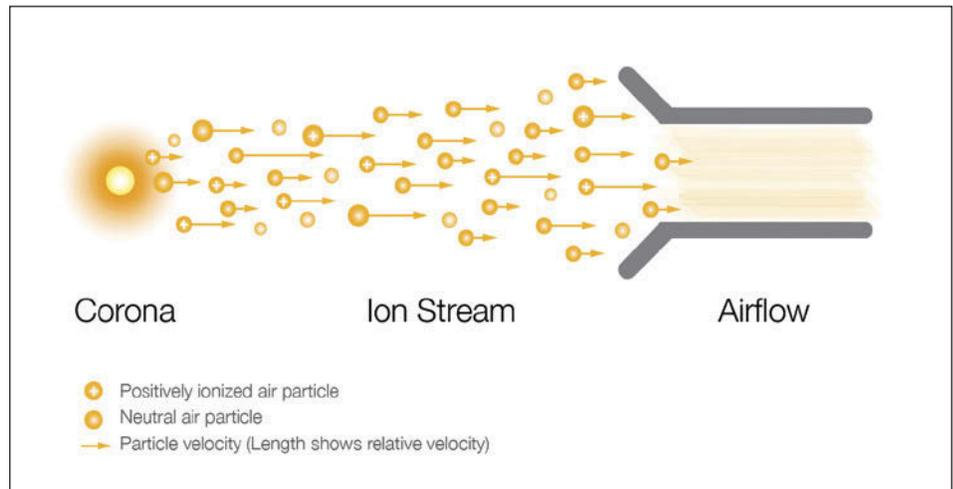
FIGURE 1: Working principle of Silent Air Cooling™.
