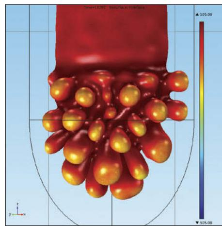
FIGURE 2: Morphological instability at the liquid-solid interface.
