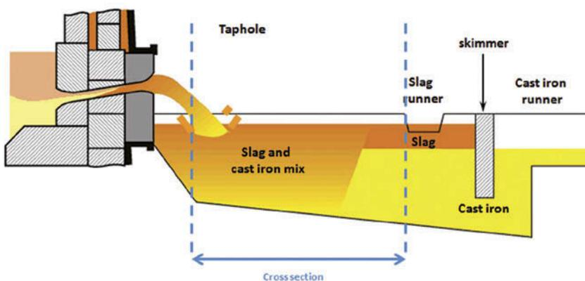
**FIGURE 1:** Molten metal exits a blast furnace (left) and travels through a runner where slag is separated from the cast iron (right). The cross-section being studied with COMSOL Multiphysics (see Figure 2) appears in the middle zone as indicated.
