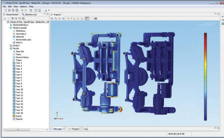
**FIGURE 2:** Dielectric stress simulation using COMSOL Multiphysics of the bypass switches (shown in the open position) and vacuum interrupter assemblies when applying a voltage across two adjacent phases. The assembly on the right is grounded.
