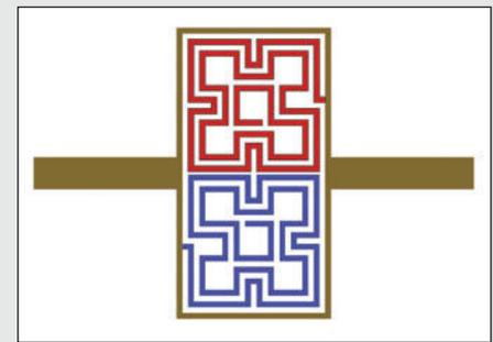
FIGURE 5: Geometry of metamaterials fractal spiral resonator: two fractal resonators are connected anti-symmetrically along the feeding line.
