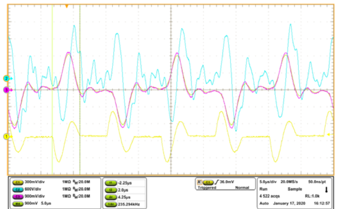
Figure 13. Winding excited by pulsed "sine" wave ( D \approx 0.4 ) Figure 14. See legends' explanation in Figure 7.
