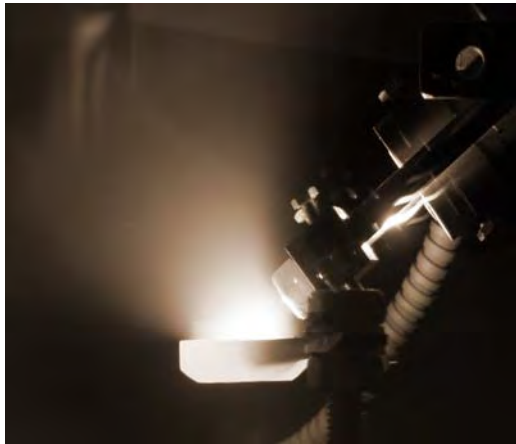
Figure 2. Photo of TVA plasma in metal vapors
