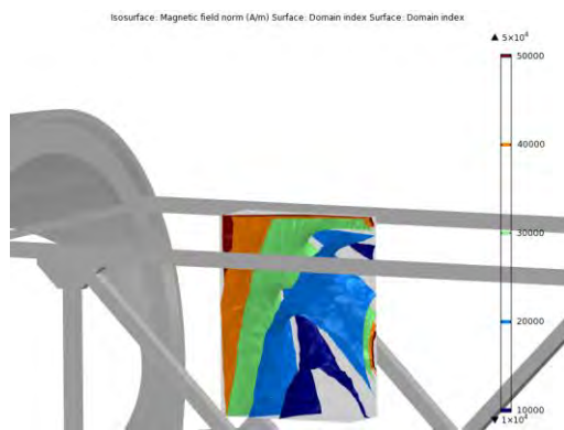
Figure 8. Isosurface plot of the magnetic field at the desired position of the panel. The result is used for determine the shielding requirements for the panel and the installations.
