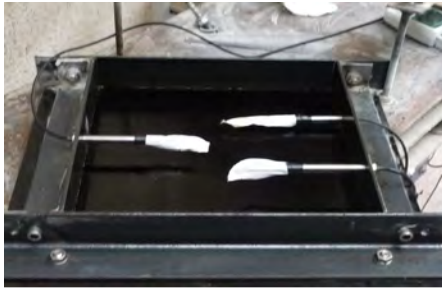
Figure 2. Instrumentation of the slab.
