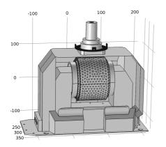
**Figure 1**: Inner parts of SF6 gas insulated VIT with air bubbles.
