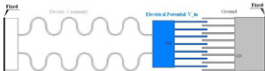
Figure 2. Schematics for comb drives with curved or rectangular serpentine flexures.
