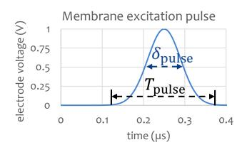
Gaussian pulse shape used  $V(t) = V_0 \cdot e^{-2\pi^2 (f_{\text{pulse}}t-1)^2}$
