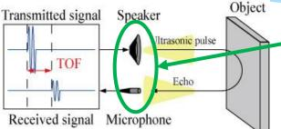
Functions combined in ultrasound transducer
