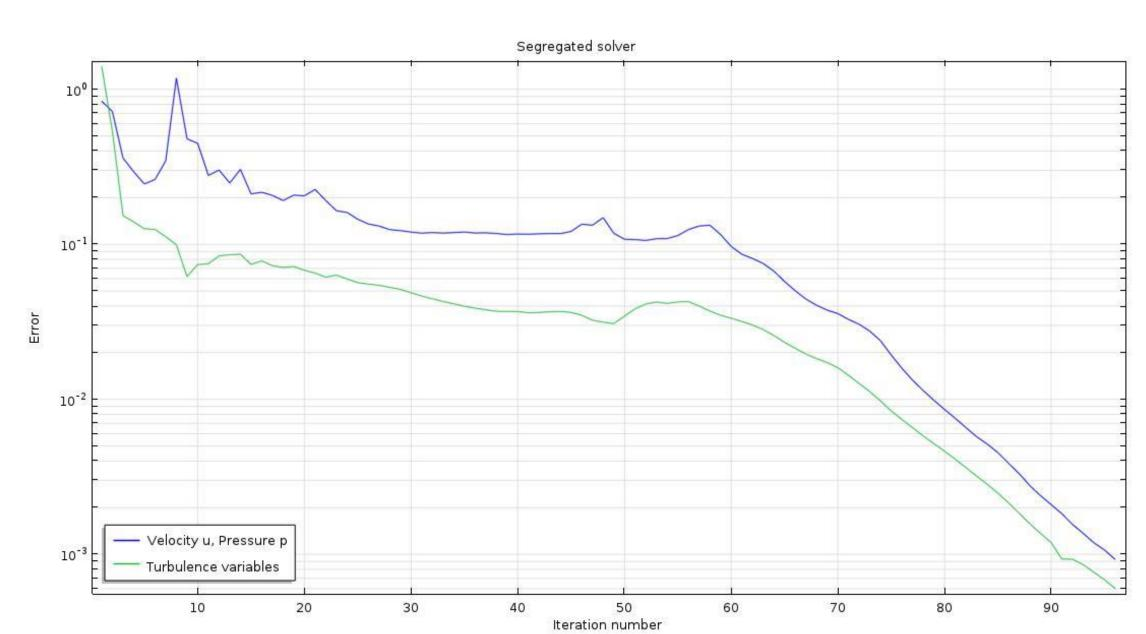
Figure 9. Velocity, Pressure and Turbulence Variables Convergence Plot
