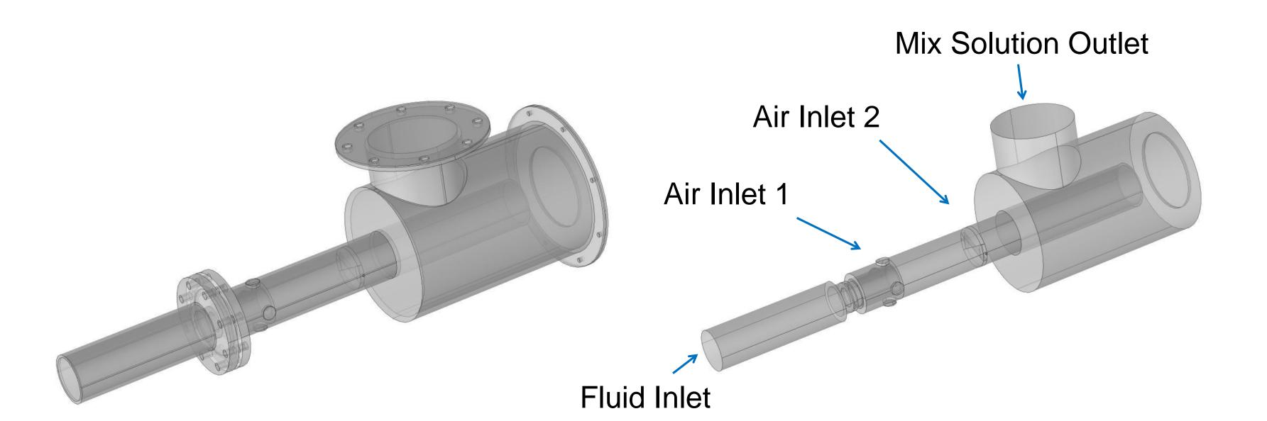
Figure 2. Foam Chamber CAD Model
