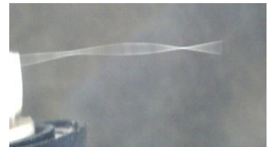
Figure 9. Third mode shape by experimental at 695 Hz
