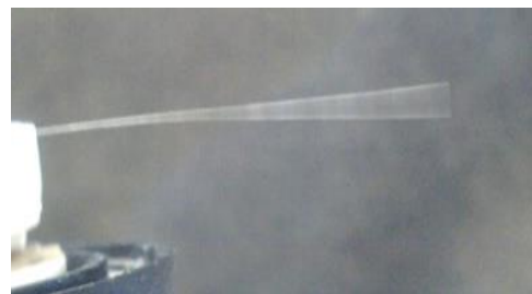
Figure 5. First mode shape by experimental at 41Hz
