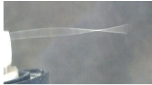
Figure 7. Second mode shape by experimental at 247 Hz
