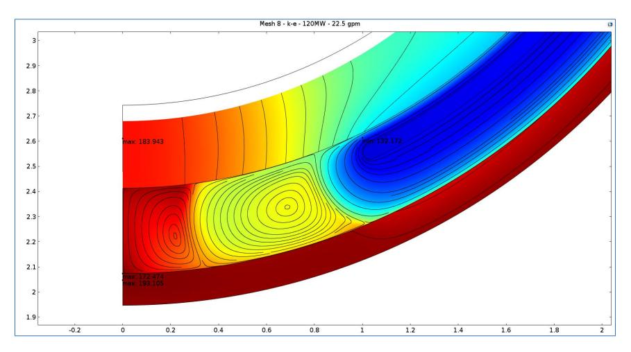
Solution View at Beam Tube Nose Detailing Temperature Contours and Velocity Streamlines for the Nominal Flow and Power Levels Using k- $\epsilon$  Turbulence Model.
