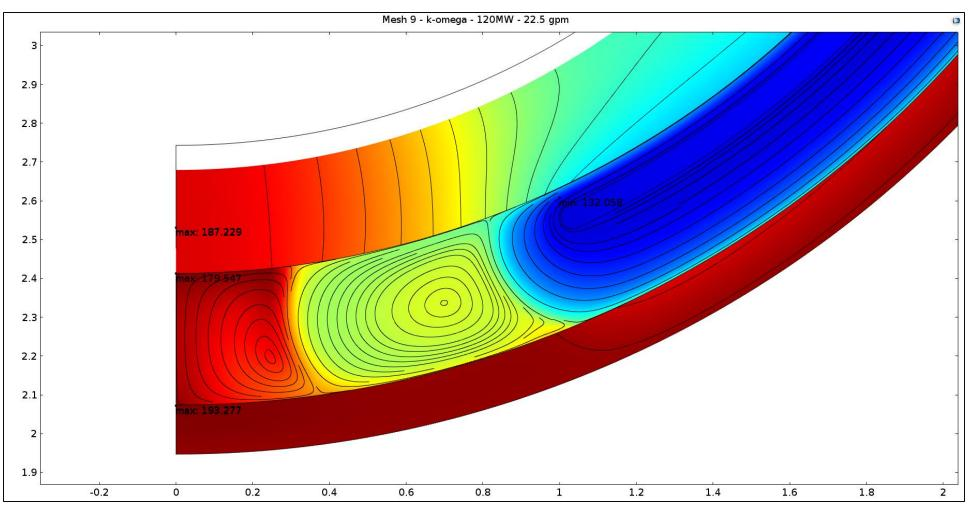
Solution View at Beam Tube Nose Detailing Temperature Contours and Velocity Streamlines for the Nominal Flow and Power Levels Using k-ω Turbulence Model.
