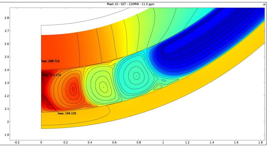
Solution View at Beam Tube Nose Detailing Temperature Contours and Velocity Streamlines for the 11.0 gpm Flow Rate and 120 MW Power Using SST Turbulence Model.
