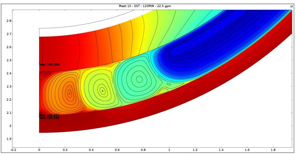
Solution View at Beam Tube Nose Detailing Temperature Contours and Velocity Streamlines for the Nominal Flow and Power Levels Using SST Turbulence Model.
