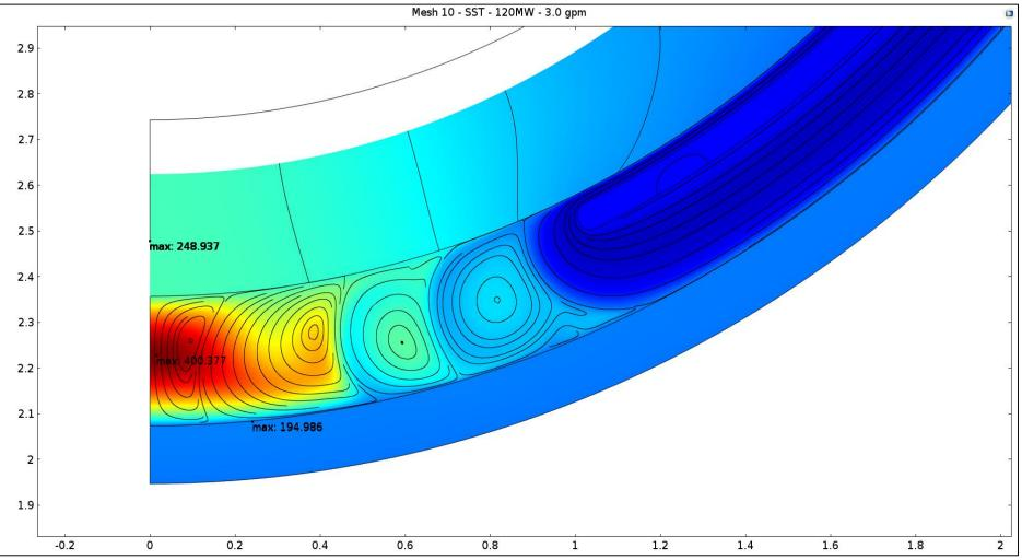
Solution View at Beam Tube Nose Detailing Temperature Contours and Velocity Streamlines for the 3.0 gpm Flow Rate and 120 MW Power Using SST Turbulence Model.
