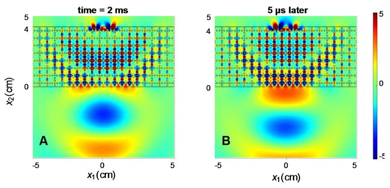
We observe one of the interesting characteristics of metamaterial: the wavevector and the group velocity have opposite directions, leading to the negative refraction and focusing.
