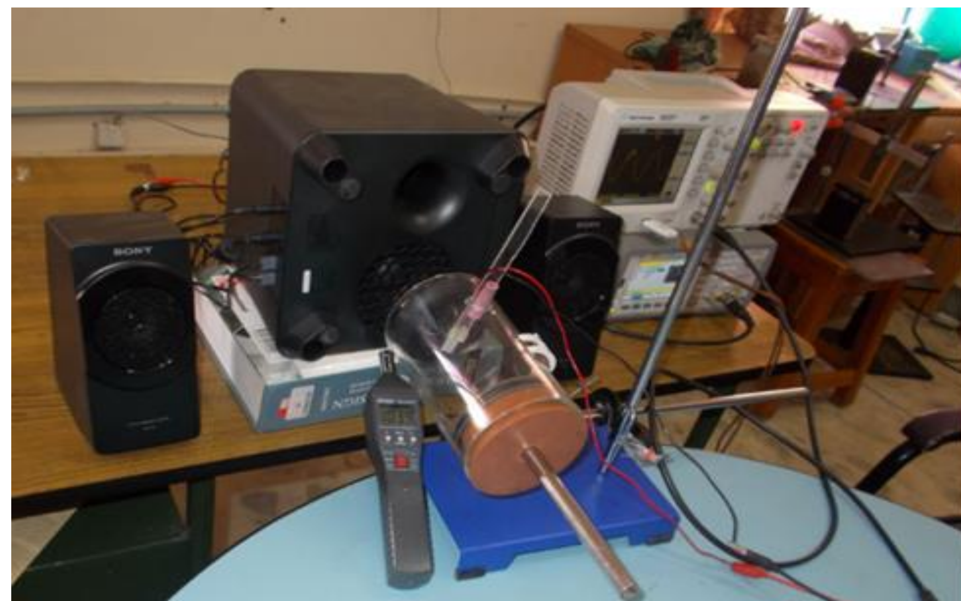
Figure 3. Experimental setup of the acoustic energy harvester.
