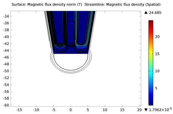
**Figure 2:** Magnetic field near the tip of the tool forming hemispherical field distribution (ball end).
