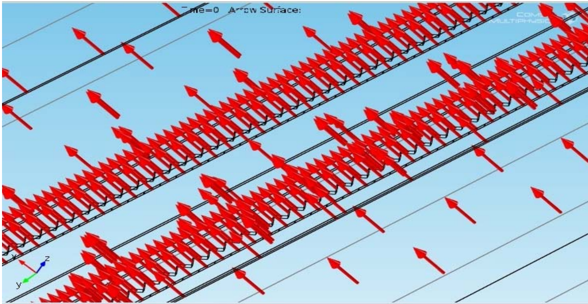
Figure 6. Electric field direction illustrating pumping mechanism
