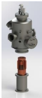
Figure 4 Chamber assembly for MAPLE with PTR cooling
