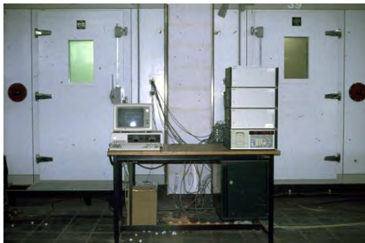
Figure 7: Hot-box device TU/e
