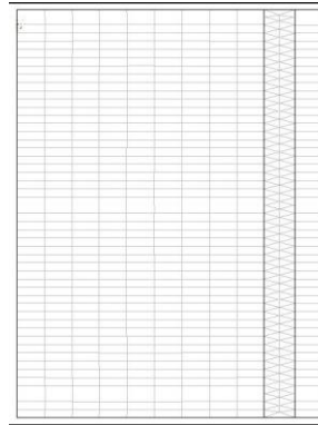
Figure 3. Mesh used consisting of a total of 700 elements.
