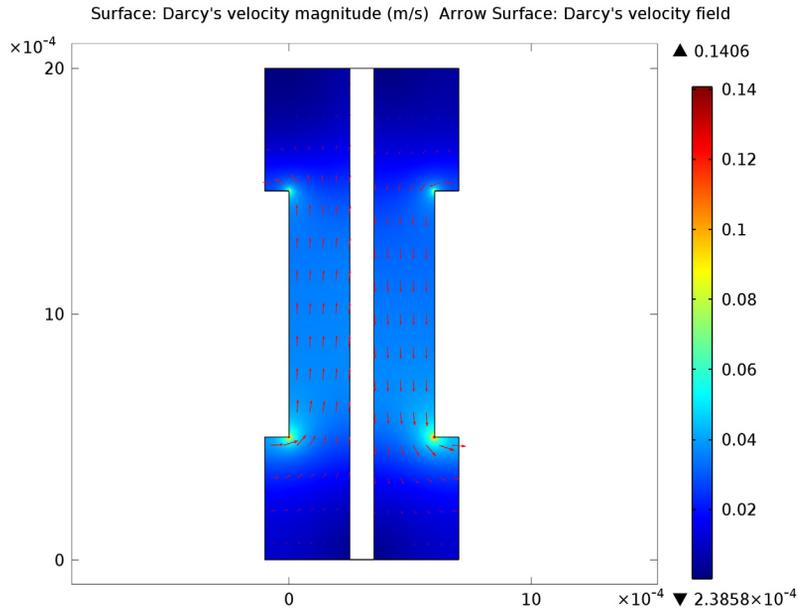
*Figure 4: Gas velocity field in the anode and cathode compartments.*
