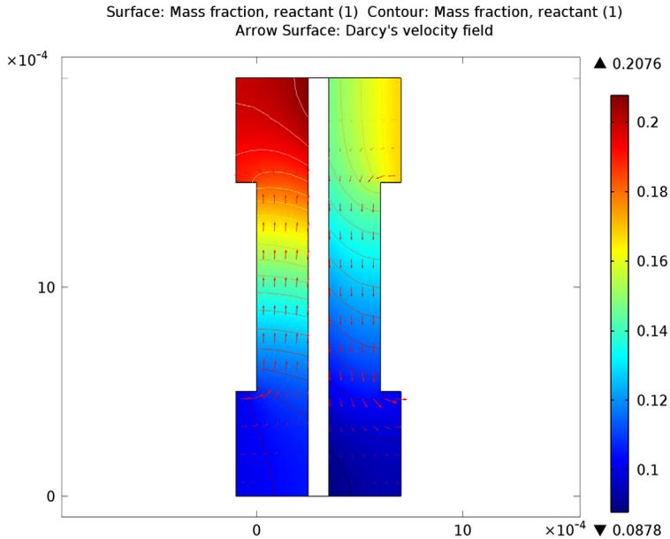
*Figure 5: Reactant mass fractions, normalized by their inlet values, on the anode side (left) and cathode side (right). The reactant in the anode is hydrogen and that in the cathode is oxygen.*
