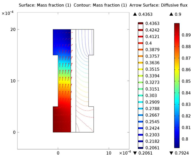
Figure 6: Water mass fraction in the anode (left, surface plot) and the cathode (right, contour plot). The arrows visualize the diffusive flux vector field on the anode side.
