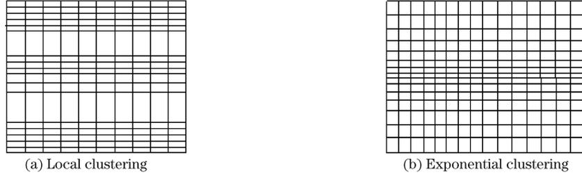
**Fig. 2** Clustering technique in mesh generation
