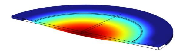
**Figure 3**: Baseline SJA displacement plot driven at 100Vrms and 207Hz (optimal frequency assuming constrained max membrane displacement to prevent interference)
