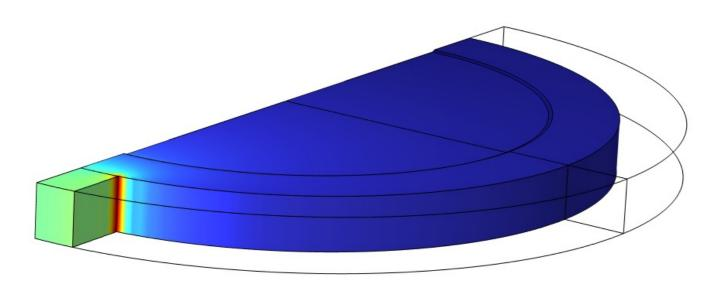
Figure 4: Optimal SJA configuration considering cavity height, orifice width and driving frequency
