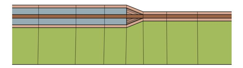
Figure 2: Internal view of the piezo bimorph membrane configuration in contact with the internal cavity air domain (green)
