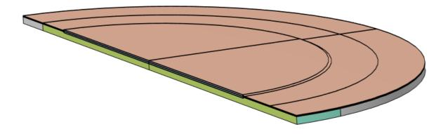
Figure 1: Symmetrical quarter model of the SJA baseline geometry
