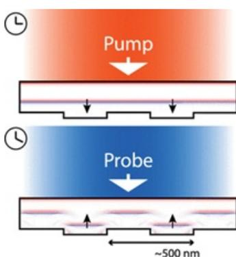
**Figure 1** : Fig 1. : Femtosecond laser pulse generates acoustic waves that diffract from buried nanostructures and are probed with a delayed pulse to reveal subsurface details.
