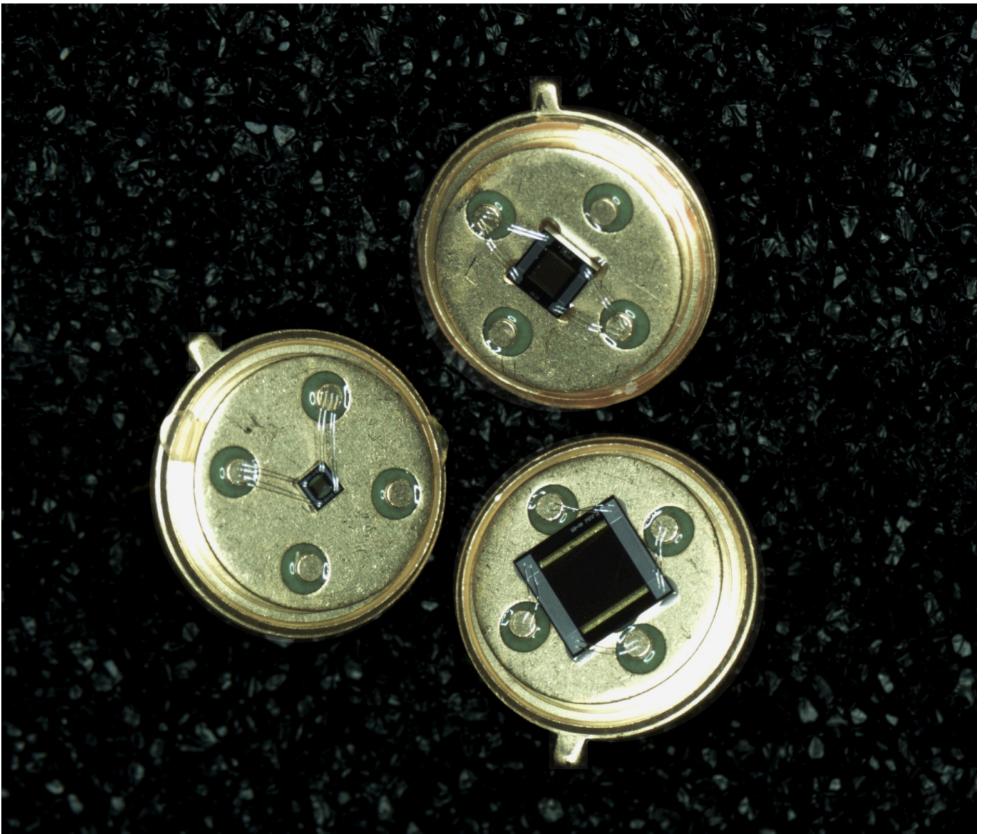
Figure 2 : Three different sizes of the MEMS-IR emitters. The large chip in the bottom right is the reference type, which served as the basis for the COMSOL model.
