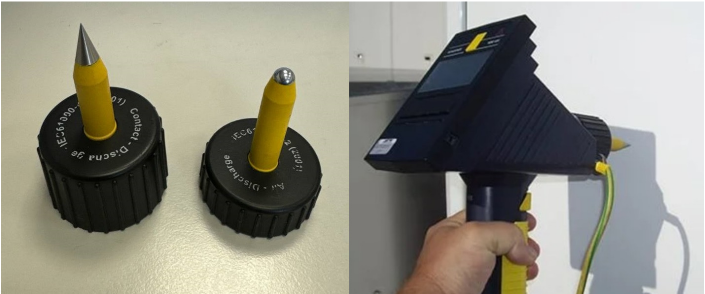
Figure 1 : NSG 435 ESD Gun with Air and Contact Finger Types
