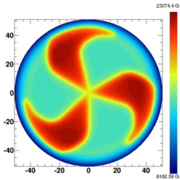
Figure 1: Simulated Magnetic field obtained for the CS-30 Cyclotron.
