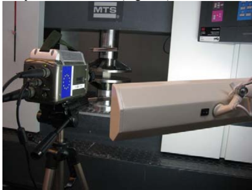
Figure 2. Testing setup comprising high speed camera observation and universal testing machine.
