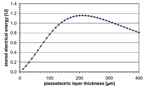
**Figure 5.** Electrical energy converted by the device as a function of piezoelectric layer thickness, when a sinusoidal vertical acceleration, with a magnitude of 0.1  $g$  and a frequency of 10 Hz, is applied to the cantilever.
