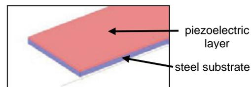
**Figure 1.** Piezoelectric converter structure.
