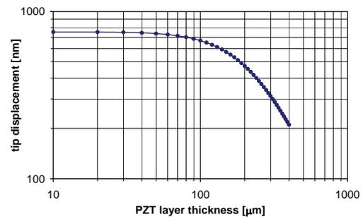
**Figure 3.** Tip displacement of the free edge as a function of piezoelectric layer thickness when a sinusoidal vertical acceleration, with a magnitude of  $0.1\ g$  and a frequency of 10 Hz is applied to the cantilever.
