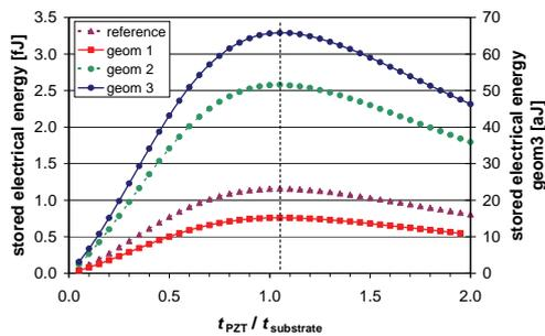
**Figure 6.** Electrical energy converted by the device as a function of piezoelectric layer thickness, for different geometries, when a sinusoidal vertical acceleration, with a magnitude of 0.1 g and a frequency of 10 Hz, is applied to the cantilever.
