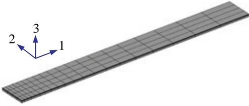
Figure 2. Piezoelectric converter mesh.
