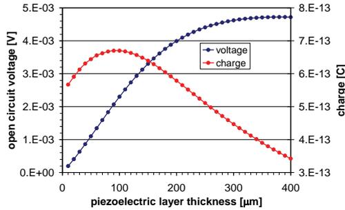
**Figure 4.** Open circuit voltage and generated charge as a function of piezoelectric layer thickness, when a sinusoidal vertical acceleration, with a magnitude of 0.1  $g$  and a frequency of 10 Hz, is applied to the cantilever.
