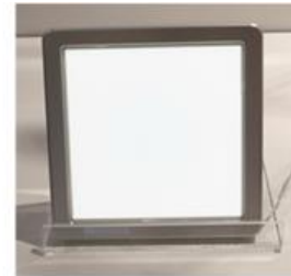
Large area OLED using new printable anode @CEATEC Japan 2012
