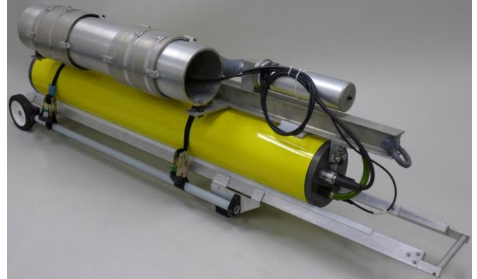
Fig. 7 Sound source system.
