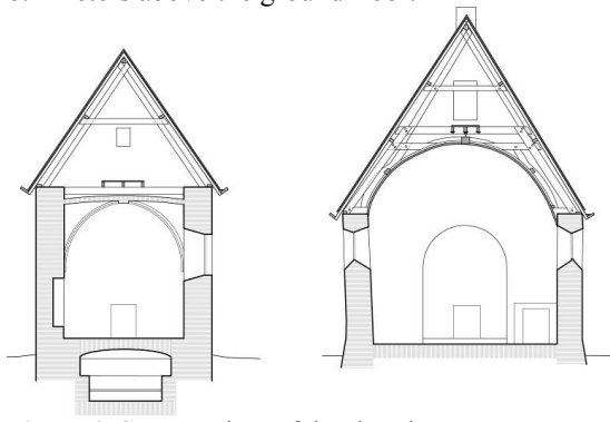
Figure 4. Cross sections of the chapel
