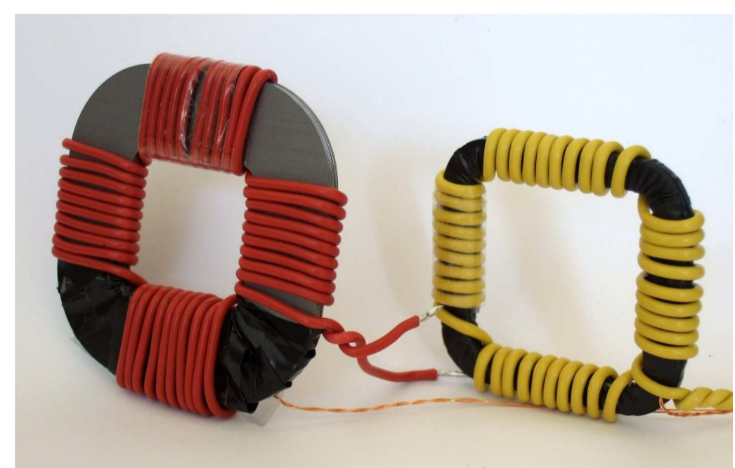
Figure 2: Transformers with laminated ring core for hysteresis measurements.
