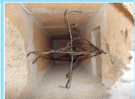
Temperature gauges distribution inside an instrumented section
