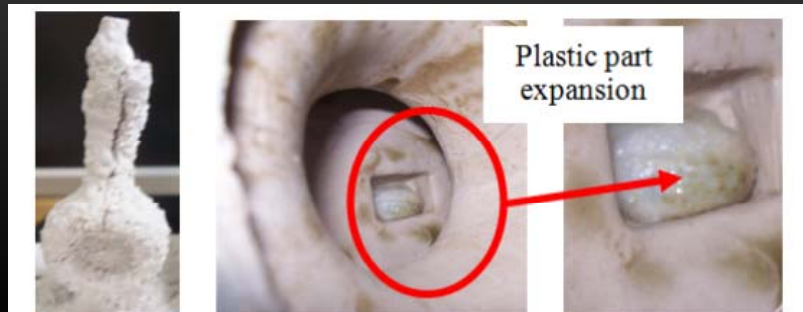
Fig. 8 Plastic material flow observed after regular De-Wax process.
