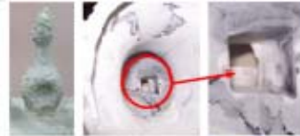
Fig. 11. Very clean ABS burn out under 1120°C without shell crack.
