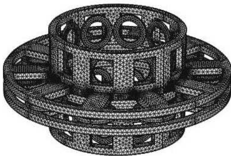
Figure 5 Model of the generator with finite element mesh (surrounding air cylinder hidden)
