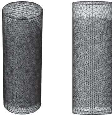
Figure 2. Coarse (left) and Extra coarse (right) meshes.
