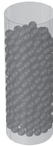
Figure 1. 400-sphere packed bed with N = 5.96 .
